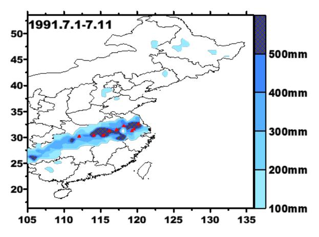
Figure. Persistent precipitation extremes, which occurred from 1 to 11 July 1991. Shadings indicate accumulated precipitation (mm), and red triangles label the stations which experienced at least three consecutive days with extreme precipitation of at least 50 mm per day.
